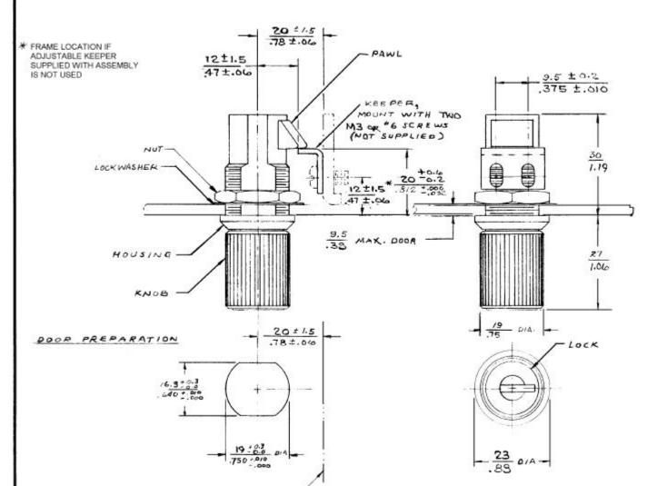
ASSEMBLY PART No. 93-10-202-10 CONSISTS OF 1 LATCH SUB-ASS'Y. 2 KEYS 1 NUT, 1LOCKWASHER & 1 KEEPER PACKED IN A PLASTIC BAG.
