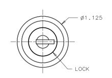
ASSEMBLY PART NO. 93-10-101-10 CONSISTS OF ONE LATCH SUB-ASSY, TWO KEYS, ONE NUT, ONE LOCKWASHER AND ONE KEEPER, PACKED IN A PLASTIC BAG.
