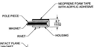
TO INSTALL REMOVE PROTECTIVE PAPER AND APPLY ASSEMBLY TO A CLEAN, DRY SURFACE
