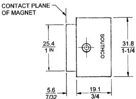
NOTES: MAGNETIC CATCHES IN GENERAL AND ADHESIVE MOUNTING ASSEMBLIES IN PARTICULAR ARE DESIGNED TO FUNCTION UNDER INTERMITTENT BREAK AWAY LOADS. DO NOT SUBJECT ADHESIVE MOUNTING ASSEMBLIES TO A CONTINUOUS LOAD.
