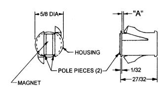
HOUSING - POLYPROPYLENE, BLACK MAGNET - BARIUM FERRITE POLE PIECES - 1010 STEEL, ZINC PLATE PER QQ-Z-325 TY.I, CL.3
