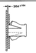
SNAP LATCH INTO HOLE IN FRAME & CLOSE DOOR
